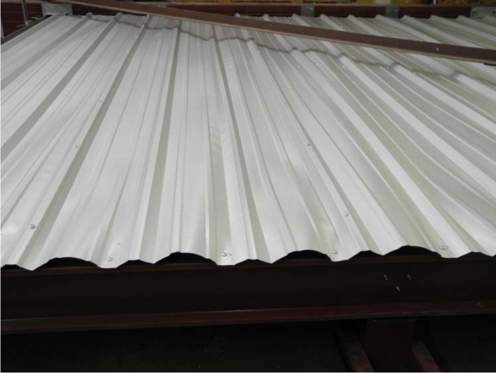
PHOTO 5 View of panel buckling in Test #1. (DSCN3183)
