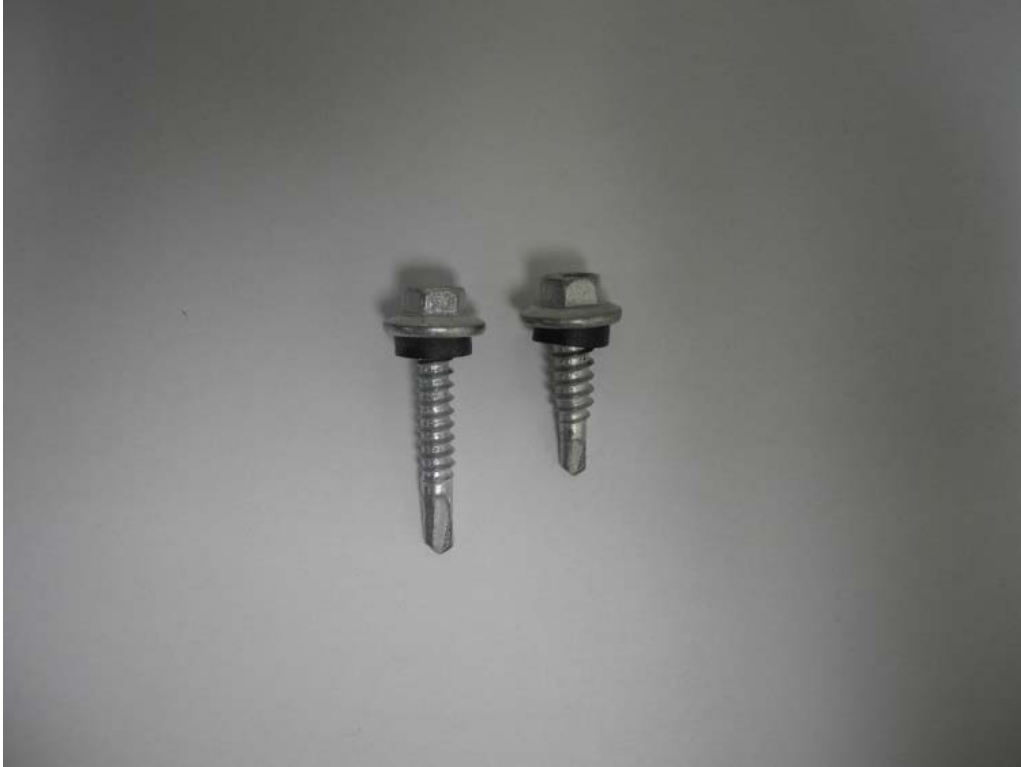
PHOTO 1 View of the panel and sidelap fasteners used in all tests. (DSCN3201)
