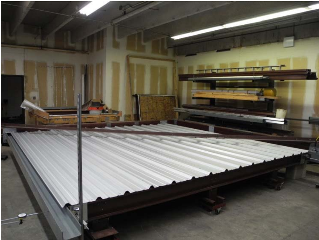
PHOTO 2 Overview of the diaphragm test setup of R-Loc panels. (DSCN3179)
