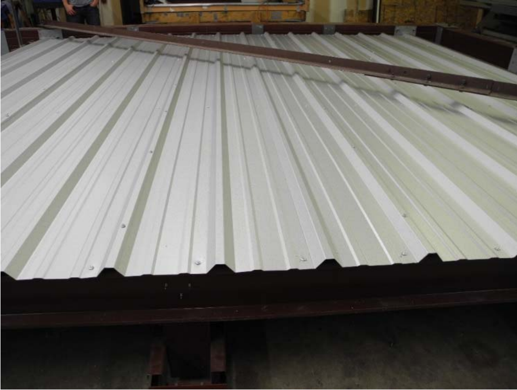
PHOTO 7 View of sidelap and panel fasteners at end and interior supports. (Test #3) (DSCN3193)
