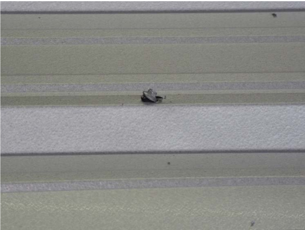
PHOTO 8 View of bearing and tilting failure of sidelap fastener in Test #3. (DSCN3199)
