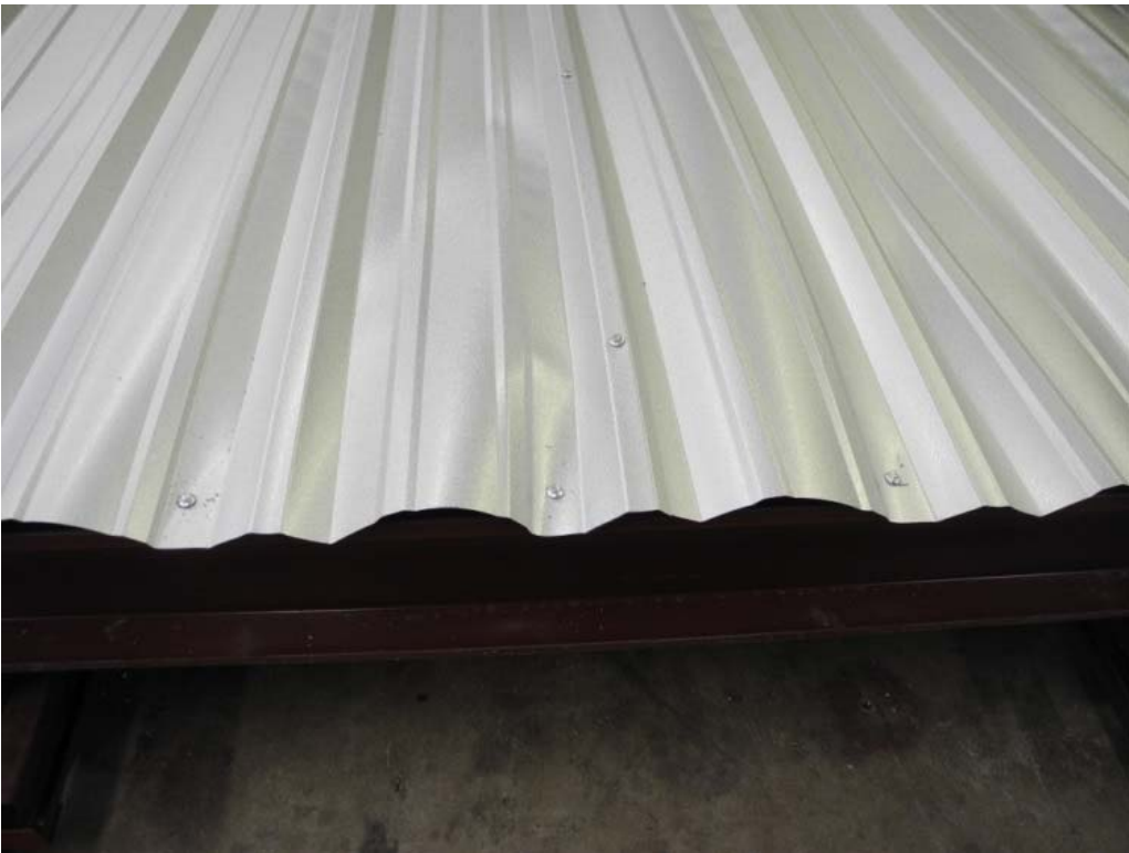
PHOTO 6 View of panel buckling in Test #2. (DSCN3189)
