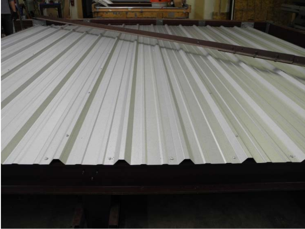
PHOTO 3 View of panel and sidelap fasteners at end and interior supports (Tests #1 & 2). (DSCN3180)
