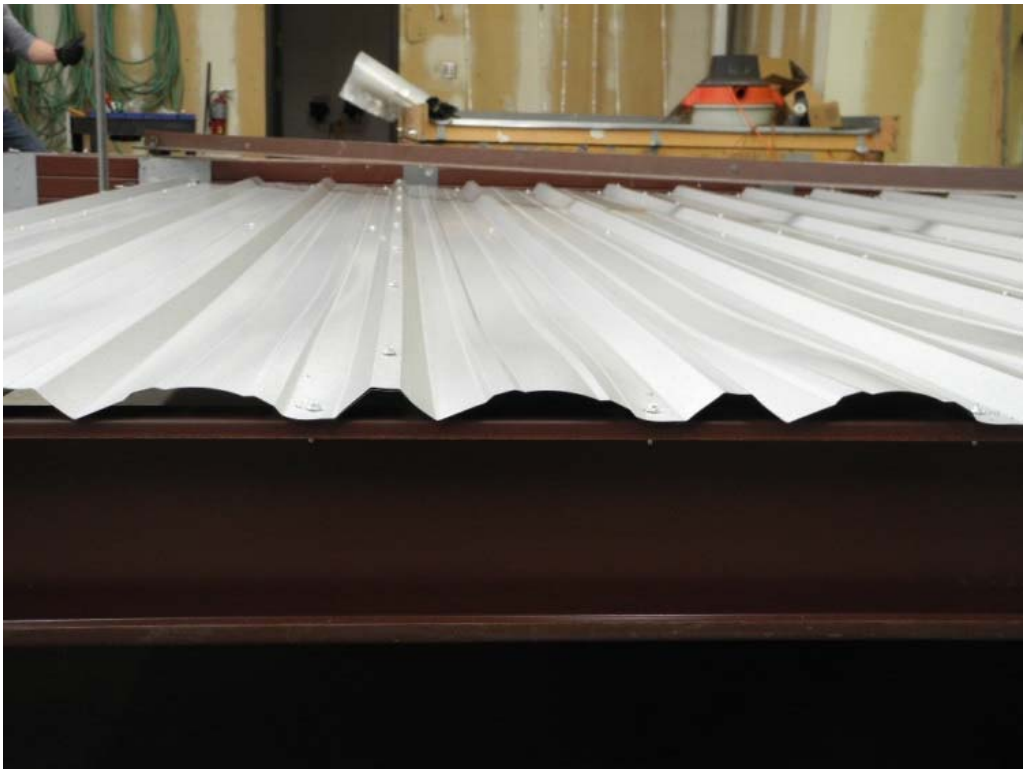
PHOTO 4 View of panel deformation under shear load in Test #1. (DSCN3181)
