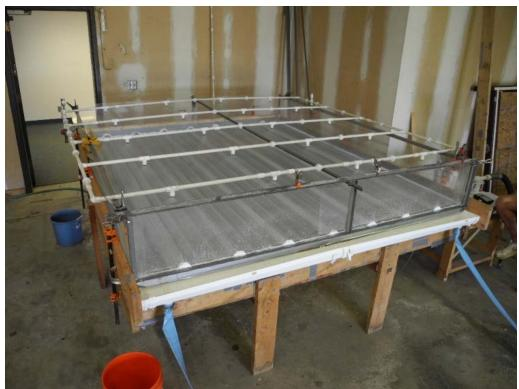
PHOTO 7 View of water spray test. (DSCN3932)
