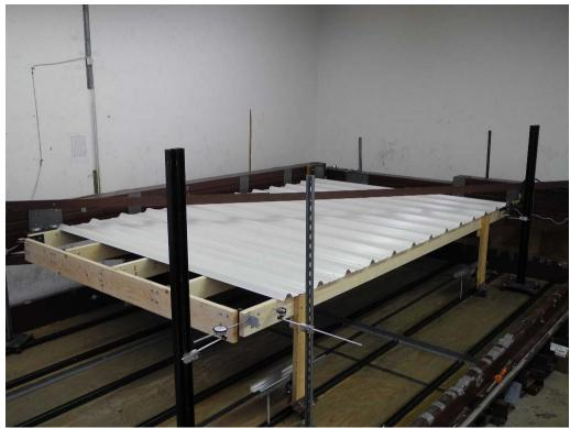
**<u>PHOTO 4</u>** Overview of the diaphragm test setup of the R-Loc panels. (DSCN0992)
