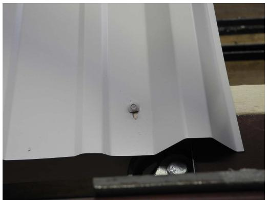
**<u>PHOTO 5</u>** View of panel slotting at fastener near the roller support in Test #1. (DSCN0999)
