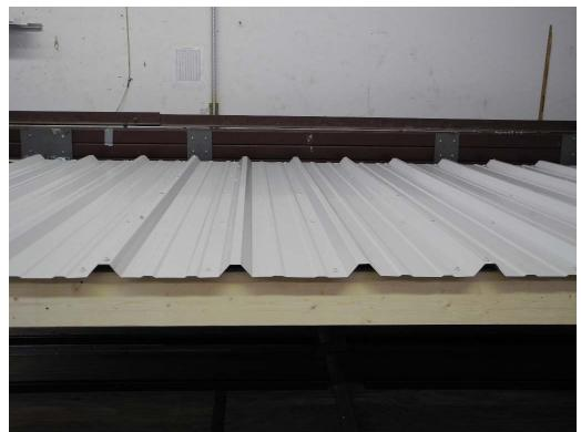
**<u>PHOTO 3</u>** View of the fasteners at end and interior supports. (DSCN1003)
