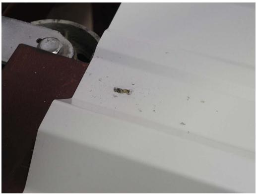
**<u>PHOTO 6</u>** View of panel slotting at fastener near the roller support in Test #2. (DSCN1011)
