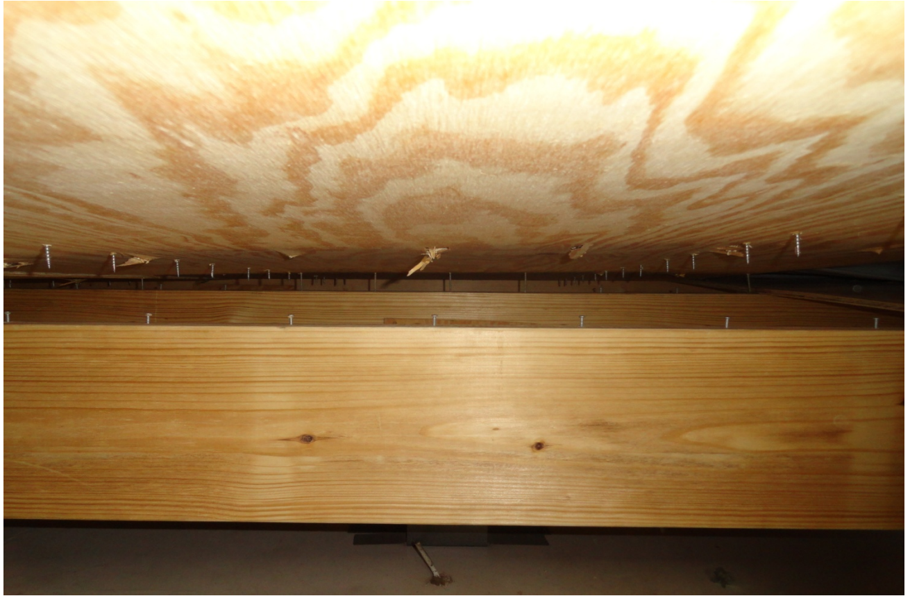
TYPICAL TEST FAILURE, PLYWOOD PULLED OFF 2X10 FRAMING
