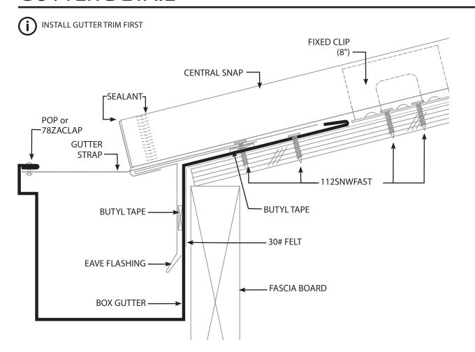
FIGURE 1. Gutter Strap
