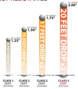
Underwriters Laboratory has developed a test (UL 2218) to evaluate the impact resistance of roofing material. This test evaluates materials by dropping a steel ball onto the roofing panel twice at the same location. The material must show no evidence of fracture, cracking, splitting, or any other failure resulting in an opening of the roofing material. The sizes of the steel balls range from 1.25" to 2.00" and are dropped twice from a height of between 12 and 20 feet.
