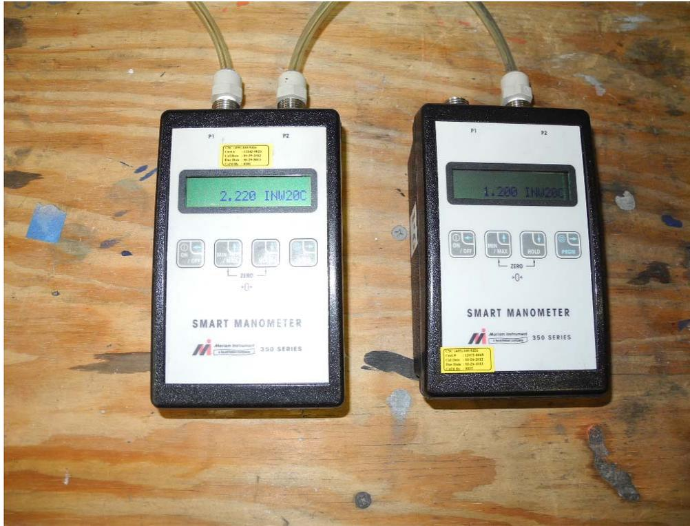
**PHOTO 7** View of flow measurements at differential pressure of 6.24 psf (equivalent to 1.2" of water). (DSCN0892)
