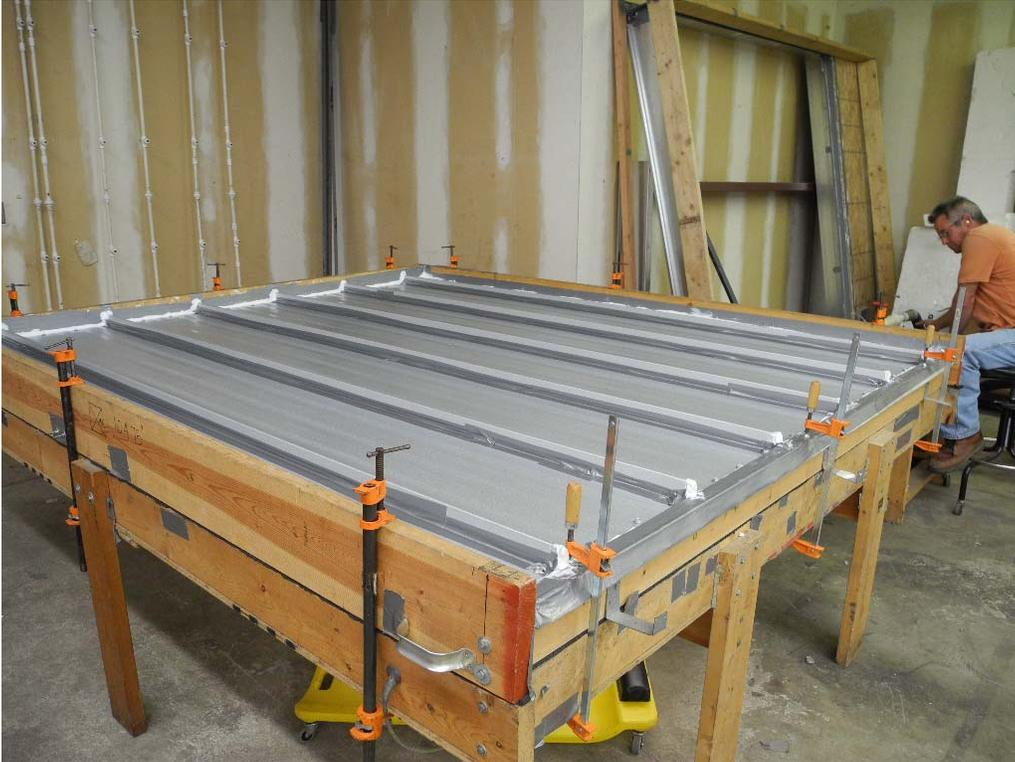
**PHOTO 5** View of the extraneous leakage measurement of the test chamber. Note the sidelap was temporarily sealed for this measurement. (DSCN0888)
