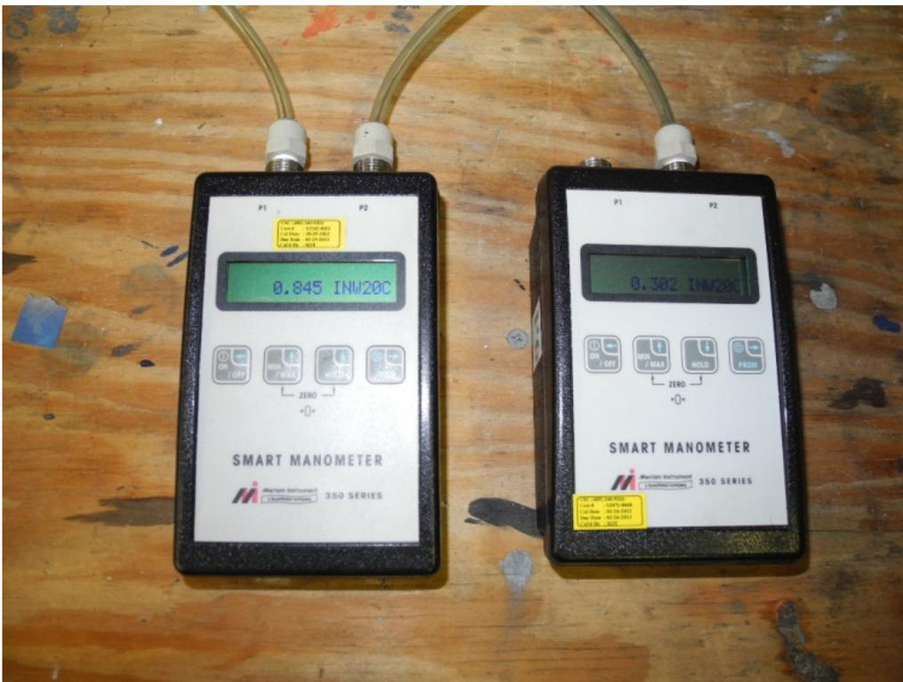
**PHOTO 6** View of flow measurements at differential pressure of 1.57 psf (equivalent to 0.302" of water). (DSCN0893)
