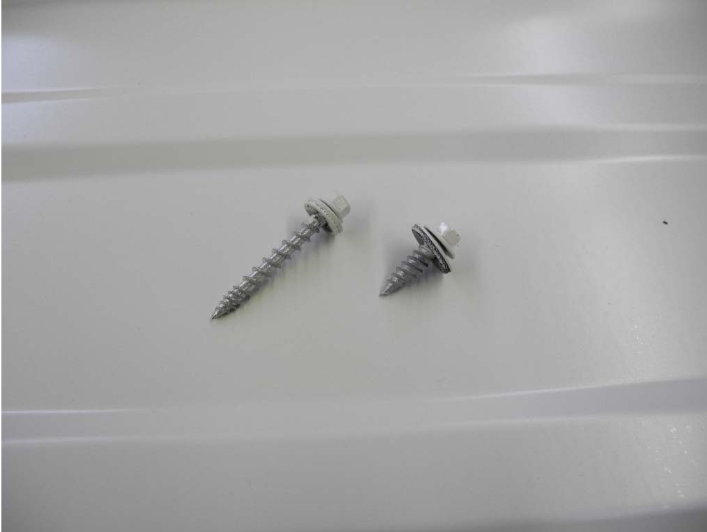
PHOTO 1 View of the structural and sidelap fasteners. (DSCN1011)
