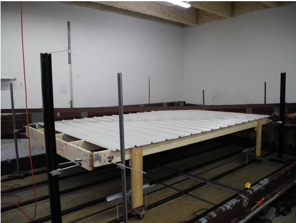
PHOTO 4 Overview of the diaphragm test setup of the Panel-Loc Plus panels. (DSCN1013)
