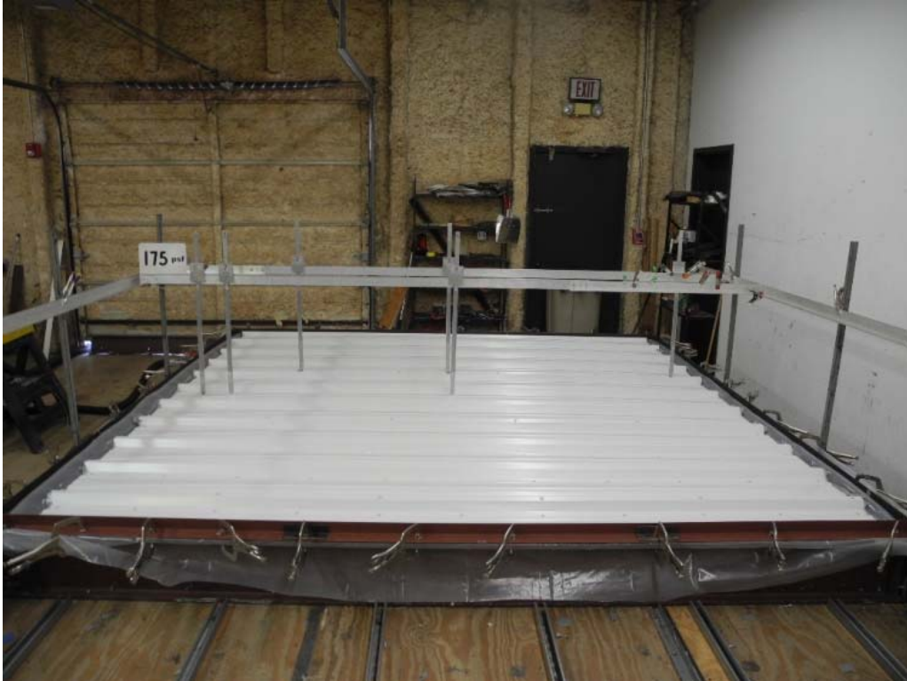
PHOTO 11 View of Test #3 at pressure of 175 psf. (DSCN6761)
