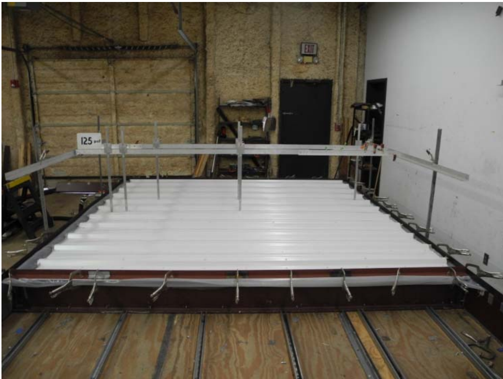
PHOTO 8 View of Test #2 at pressure of 125 psf. (DSCN6750)
