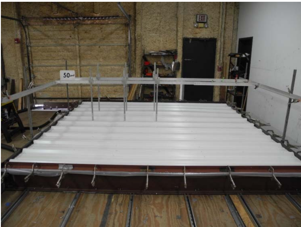
PHOTO 4 View of Test #1 at pressure of 50 psf. (DSCN6743)
