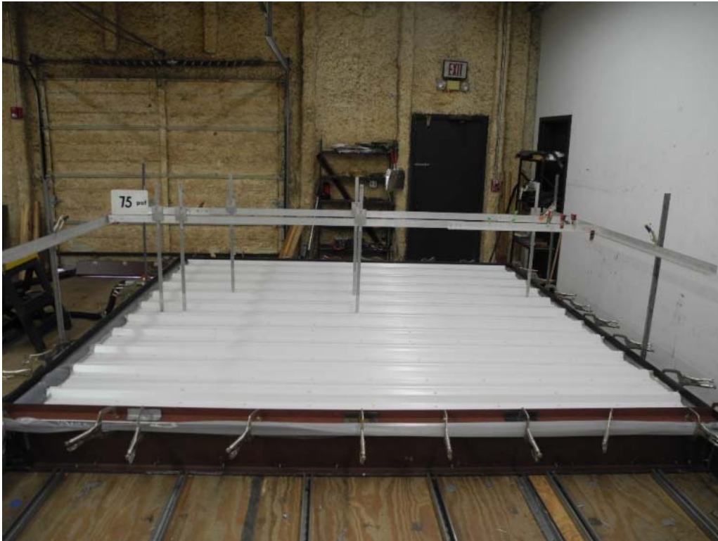
PHOTO 7 View of Test #2 at pressure of 75 psf. (DSCN6748)
