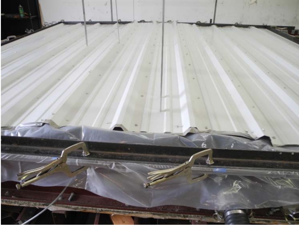
PHOTO 9 View of Test #2 at failure. The failure mode was the panel fastener pullout. (DSC00162)
