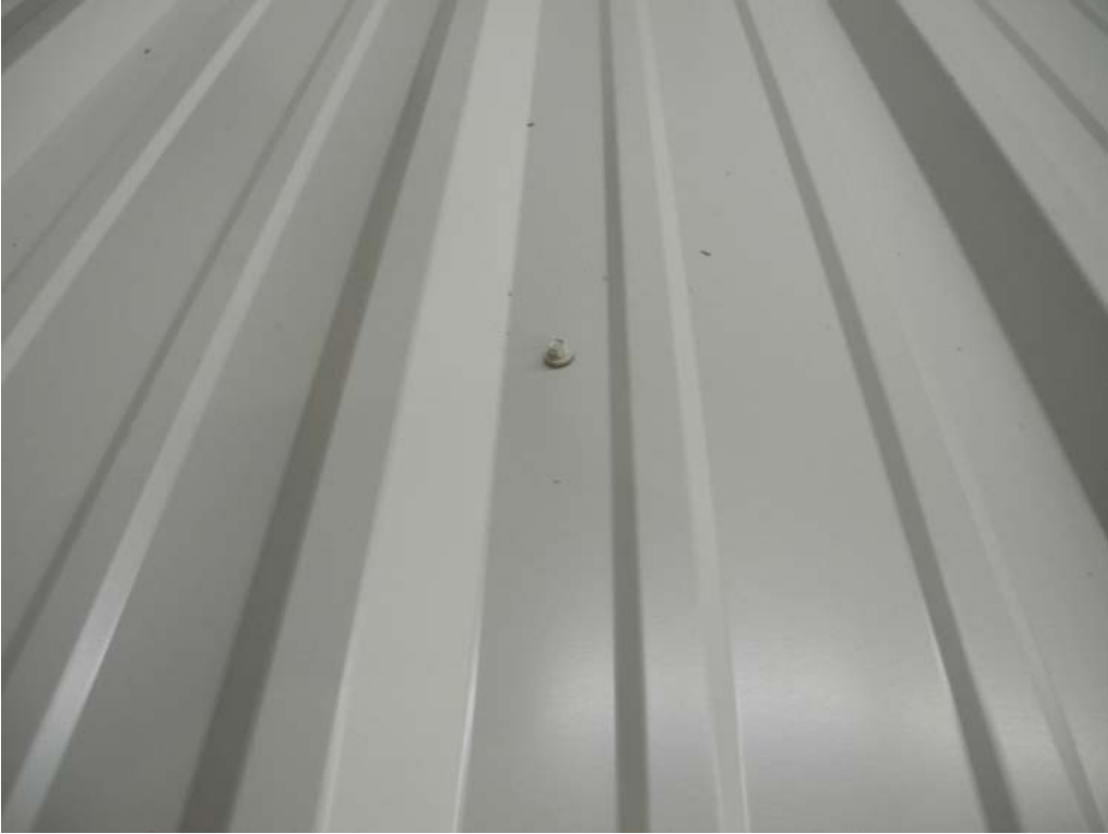
PHOTO 5 View of Test #1 at failure. The failure mode was the panel fastener pullout. (DSCN6744)
