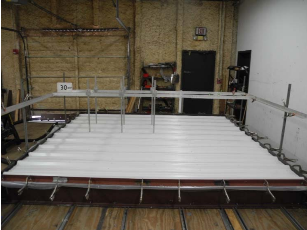
PHOTO 3 View of Test #1 at pressure of 30 psf. (DSCN6741)
