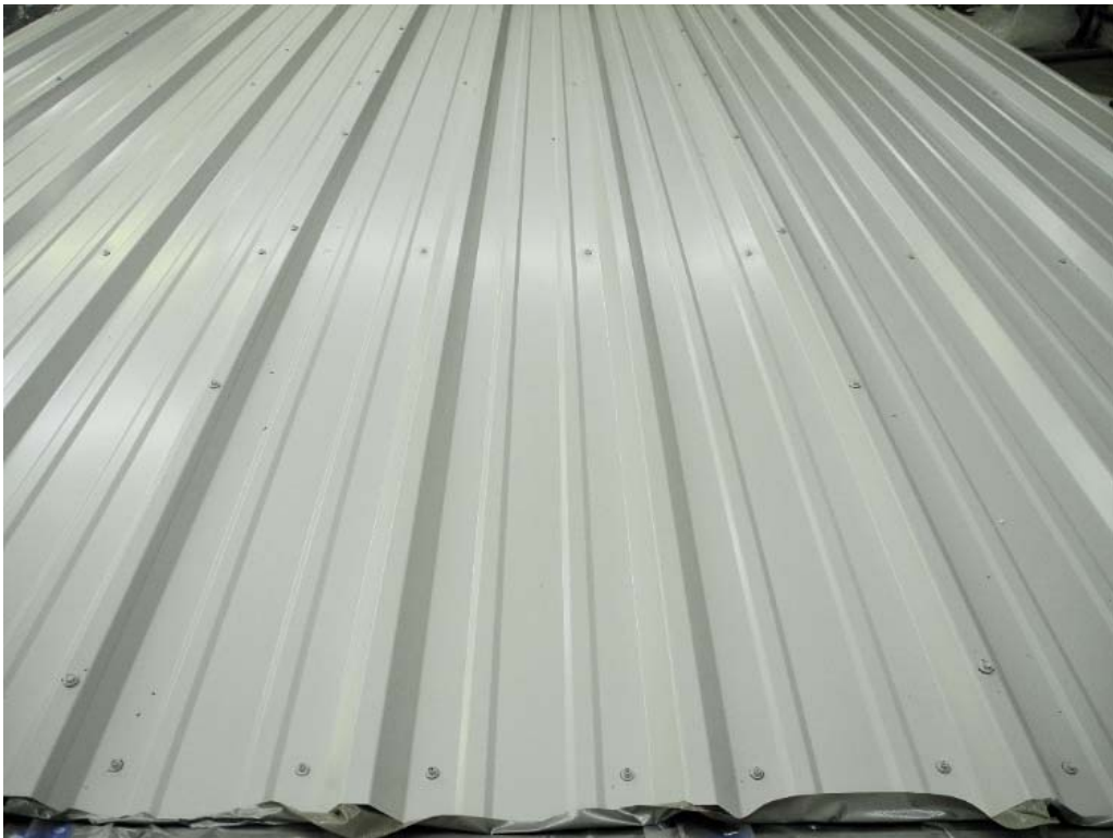
PHOTO 2 View of 26 ga. R-Loc panel fastening at panel ends and interior (Test #1). (DSCN6736)
