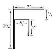
For Panel-Loc Plus™ as soffit
