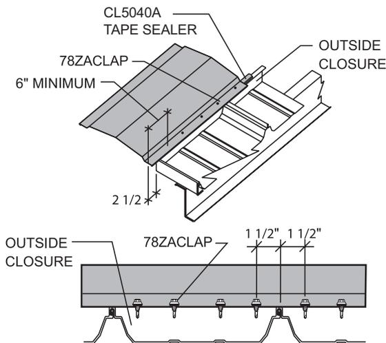
Install the ridge flashing starting and ending 2 1/2" outside the steel line. Fasten the ridge flashing to the outside closures with 78ZACLAP. Install a fastener 1 1/2" from panel seam on both sides of panel. Install additional fasteners directly above minor ribs of panel. Four fasteners are required at each panel. Leave 6" unfastened on each end to allow for the rake trim to be installed later. **DO NOT FASTEN THROUGH THE LOCK OF THE STANDING SEAM.**
