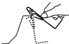
• Position the clip over the male leg of the panel as shown, and rotate clip downward.
