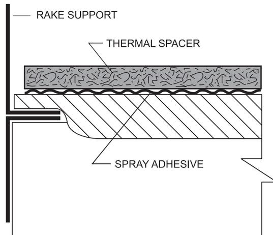
Using spray adhesive, (not by CSMI) adhere the thermal spacer to the insulation. The thermal spacer increases the insulation capacity along the purlins.
