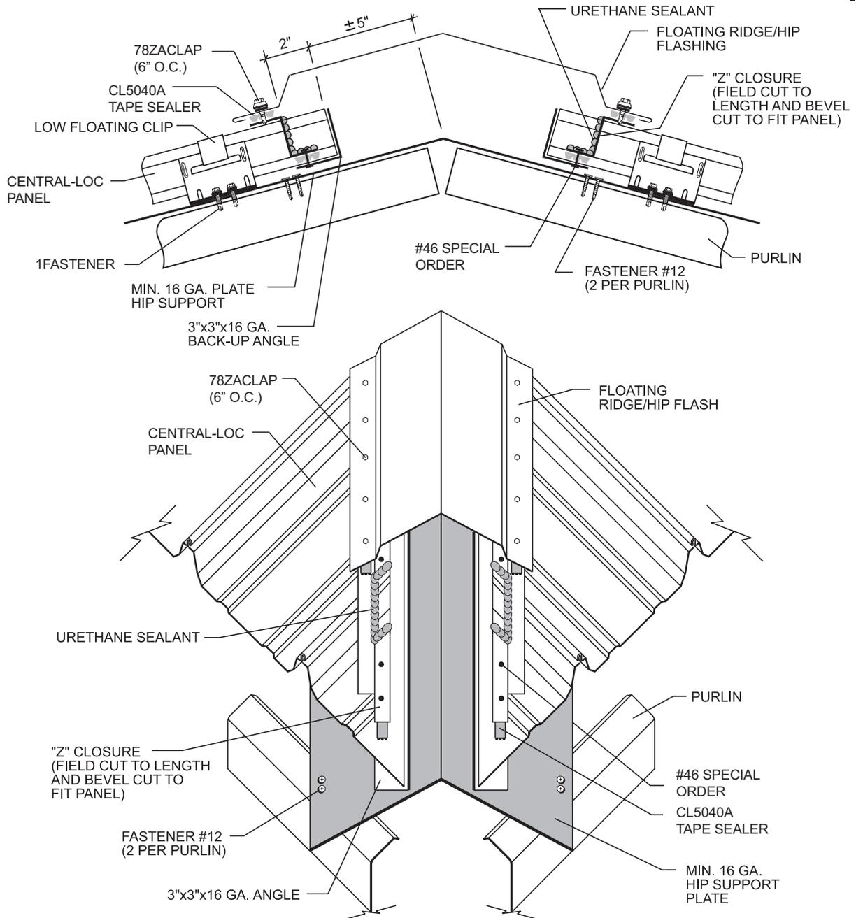
All trapezoidal panels are extremely difficult to install at hips and valleys in a weathertight manner. The use of these details should only be attempted by installation crews that are highly experienced.
