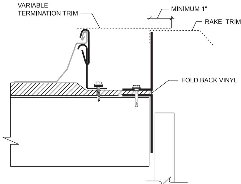
If the panel ends 2"- 4" away from the rake support due to an out-of-square condition or other factors, simply install the panel clips. This system allows for the roof to be trimmed in the high.
