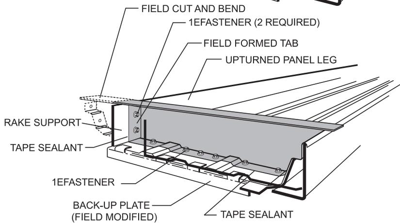
The final outside closure on the last panel may require field modification. A tab should be formed by the web of the outside closure for attachment to the upturned leg of the roof panel (field formed). This tab should be attached to the panel and angle with 1EFASTENER (2 required).
