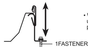
• When properly positioned, the vertical legs of the upper and lower sections of the clip will be 90° to the purlin flange pointed upward, as shown.
