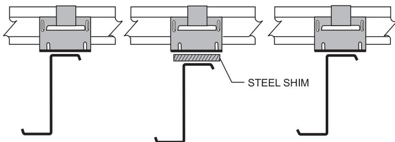
Avoid "stair-stepping" of the panels at the eave. This will cause problems engaging back-up plates at the endlap and ridge. This also will create the need to warp the cinch strap (if used) over the high rib forcing it to align with the holes in the adjacent panel.
