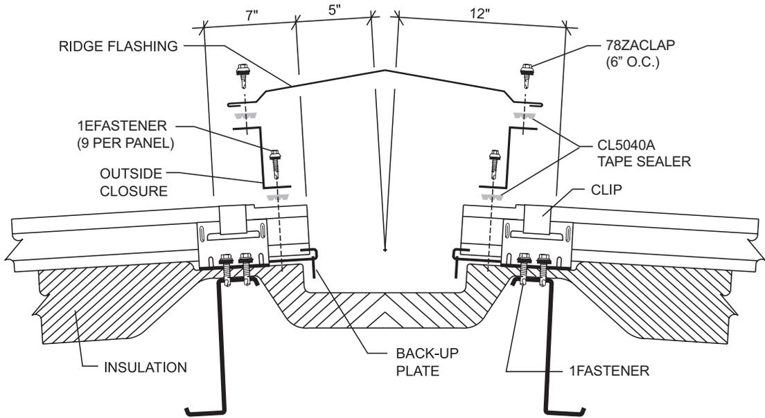
Install the ridge flashing starting and ending 2" outside the steel line. Fasten the ridge flashing to the outside closures with 78ZACLAP. Install a fastener 1" from panel seam on both sides of panel. Install additional fasteners directly above minor ribs of panel. Four fasteners are required at each panel. Leave 6" unfastened on each end to allow for the rake trim to be installed later. DO NOT FASTEN THROUGH THE LOCK OF THE STANDING SEAM.
