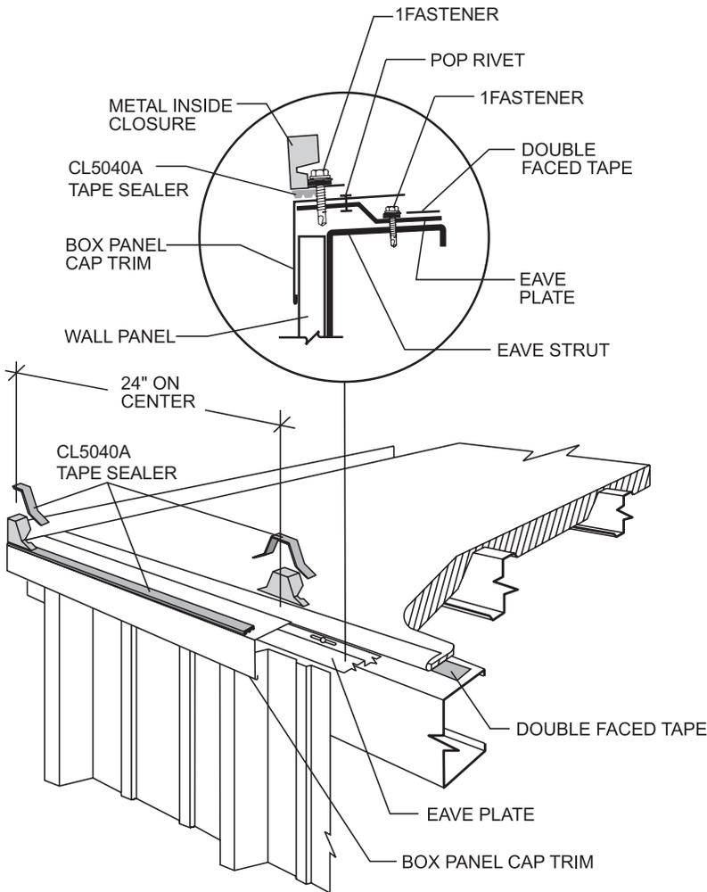
The fiberglass insulation must not interfere with the CL5040A tape sealer which provides a positive seal at the eave.
