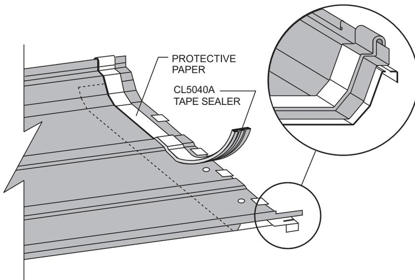
Install CL5040A tape sealer over prepunched holes. Be sure to place the tape sealer over the male leg. **DO NOT REMOVE THE PROTECTIVE PAPER AT THIS TIME, EXCEPT AT THE MALE LEG.**
