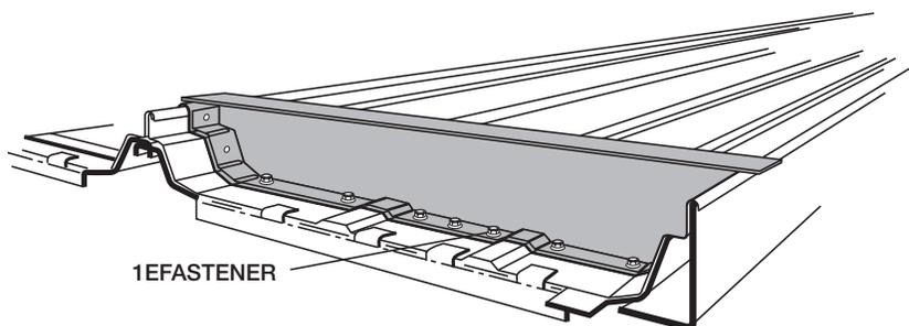
Push the other end of the outside closure into position and align the holes with the awl. Remove the awl and install 1EFASTENER in all remaining holes except for the hole at the panel seam. **Do not install the panel seam fastener at this time.**
