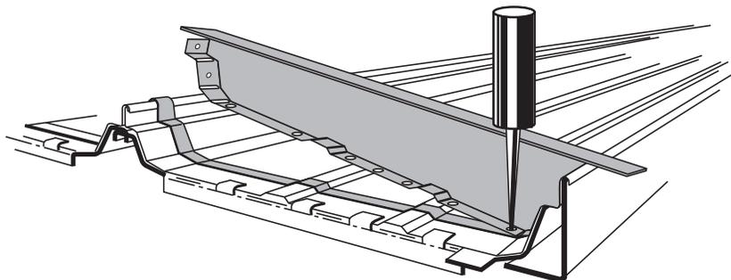
protective paper from tape sealer. Apply tape sealer to the ridge panel just installed. Be sure to seal to the mastic on the previous panel.
